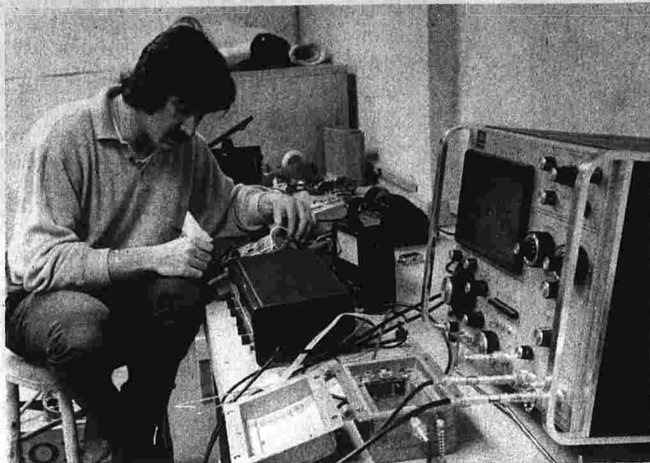
Carlos Calliva, a technical staffer at Greater Hartford CATV Inc., uses electronic test equipment to align a cable television amplifier.
