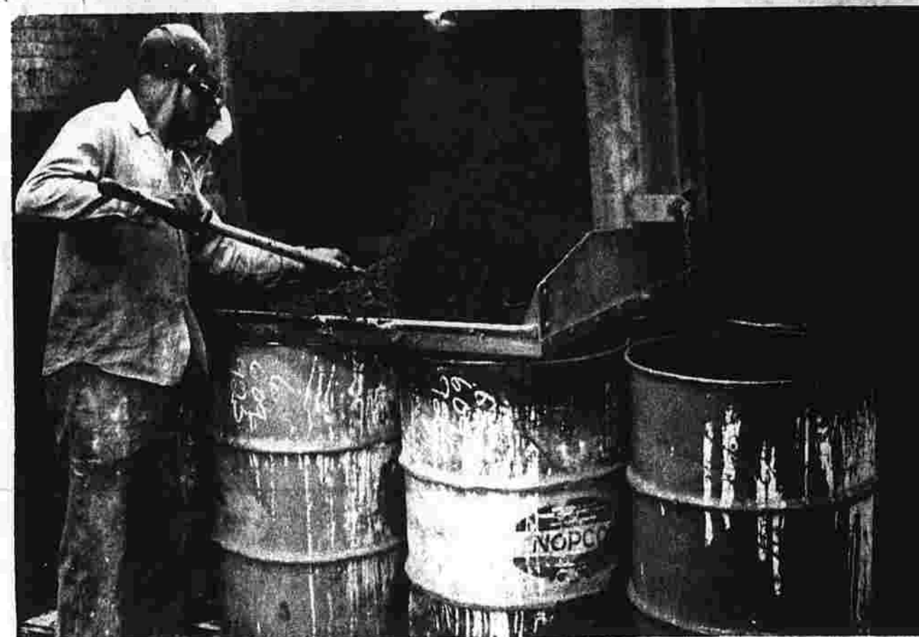
Fibers of cotton or wood, according to the needs of the product, are being combined with plastic material by Herbert Lawrence, kneader operator, at Rogers Corp.
