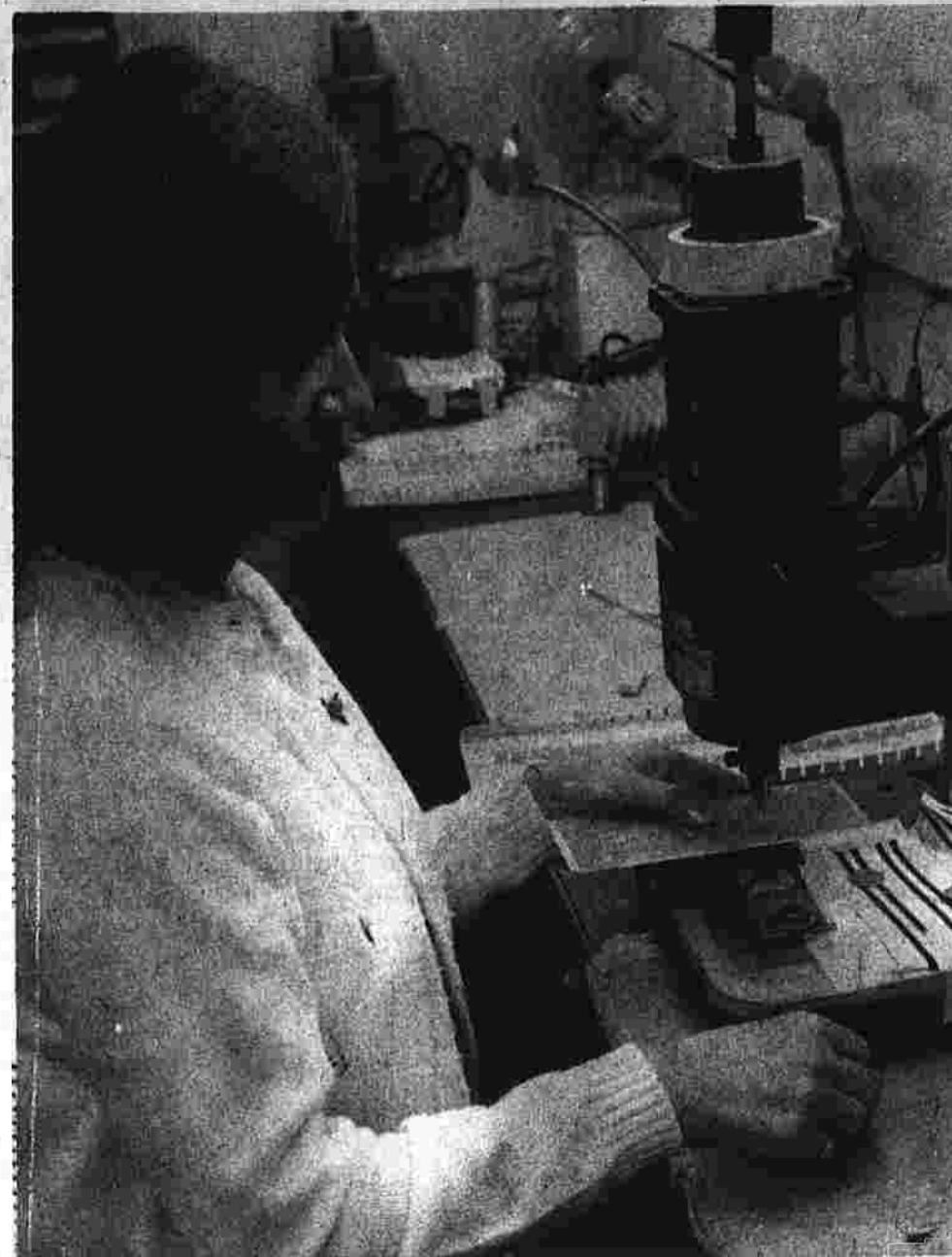
Edith Dunn begins to drill printed circuit board in the hardware department of Multi-Circuits, Inc., which makes the boards to customer specifications.
