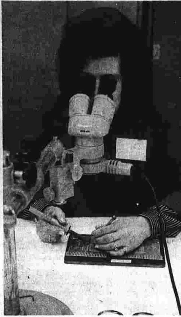
Accuracy counts in this circuit-soldering operation, so Julie Guimond uses a stereo microscope to see what she's doing. She is employed by Brand-Rex Co. of Progress Dr., one of Manchester's newest industries.
